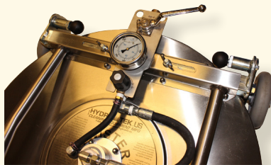
Pressure adjustment with gauge and water supply on/off ball valve on deck.
